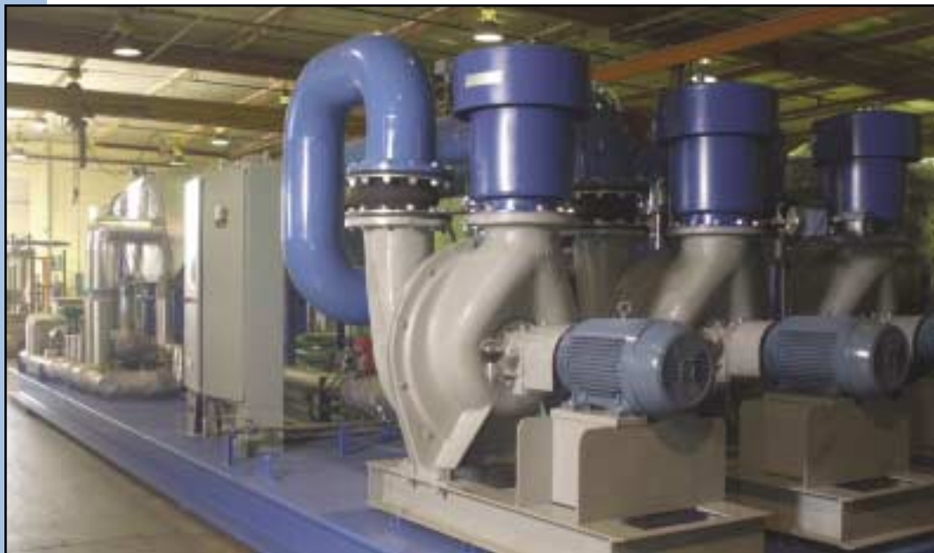
THE BUSINESS END: Ammonia Flow Control Unit (AFCU) for 1850 lb/hr U2A system ready to leave Wahlco's Santa Ana Facility. Designed for tight quarters, this AFCU skid will be nestled between ducts on the sides and platforms top and bottom.
